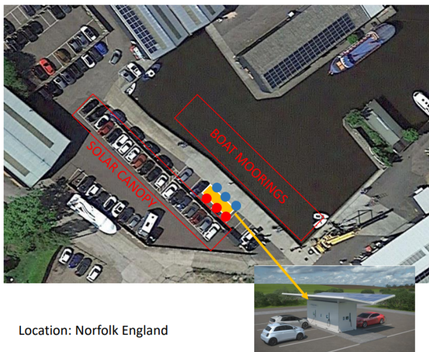
Figure A5.5: Boatyard solar augmented dual purpose EV/MEV charging station
