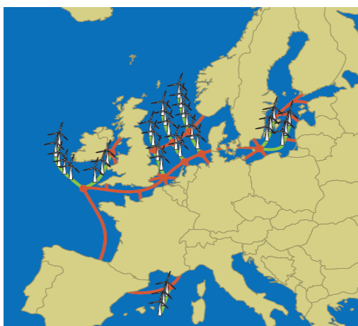
Fig. 20. Airtricity’s 10GW Foundation Project will connect wind generated electricity through an HVDC network to the UK, Germany and the Netherlands as the first phase of a Europe-wide network. Source: Airtricity, 2006.
